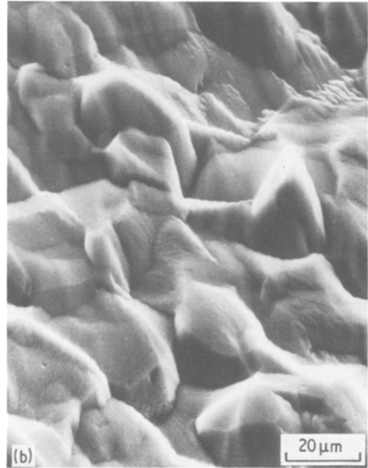
Figure 14 Titanium surface topography after natural texturing for 240 min at an accelerating voltage of 7 kV and at various incidence angles: (a) 0 rad, (b) 0.78 rad, (c) 1.05 rad, (d) 1.22 rad, (e) 1.4 rad.
