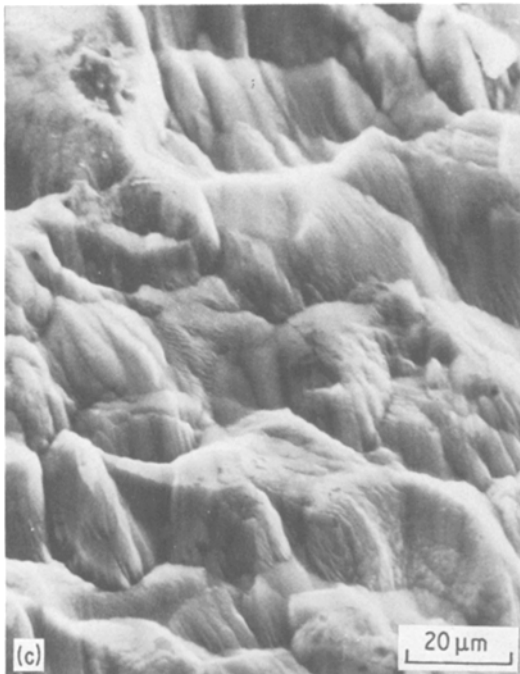
Figure 14 Titanium surface topography after natural texturing for 240 min at an accelerating voltage of 7 kV and at various incidence angles: (a) 0 rad, (b) 0.78 rad, (c) 1.05 rad, (d) 1.22 rad, (e) 1.4 rad.
